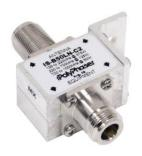
POLYPHASER 10-1000 MHz general coverage bulkhead mnt. protector. 50,000 amps surge. 220uJ throughput energy. Power based on freq. N male on equipment port. Used on the RF Antenna lines between 7/8" Coax and ½" Jumper
